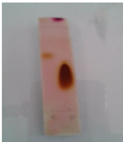
Fig.5.1 TLC plate for Benzyl Alcohol before Column Chromatography.
