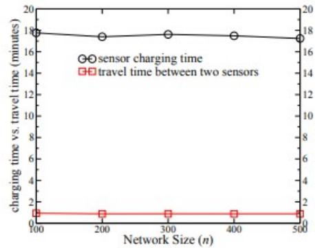
Fig sensor charging time vs. charger travel time by algorithm
