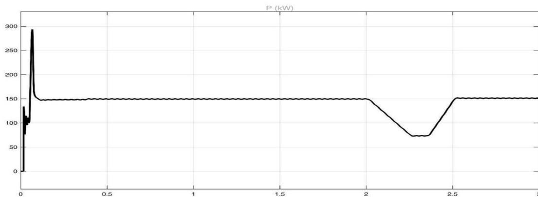
Fig 6: Output power of the grid by using Z-source converter
