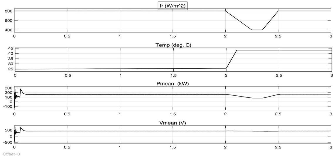
Fig 5: effect of irradiance and temperature to the power of grid
