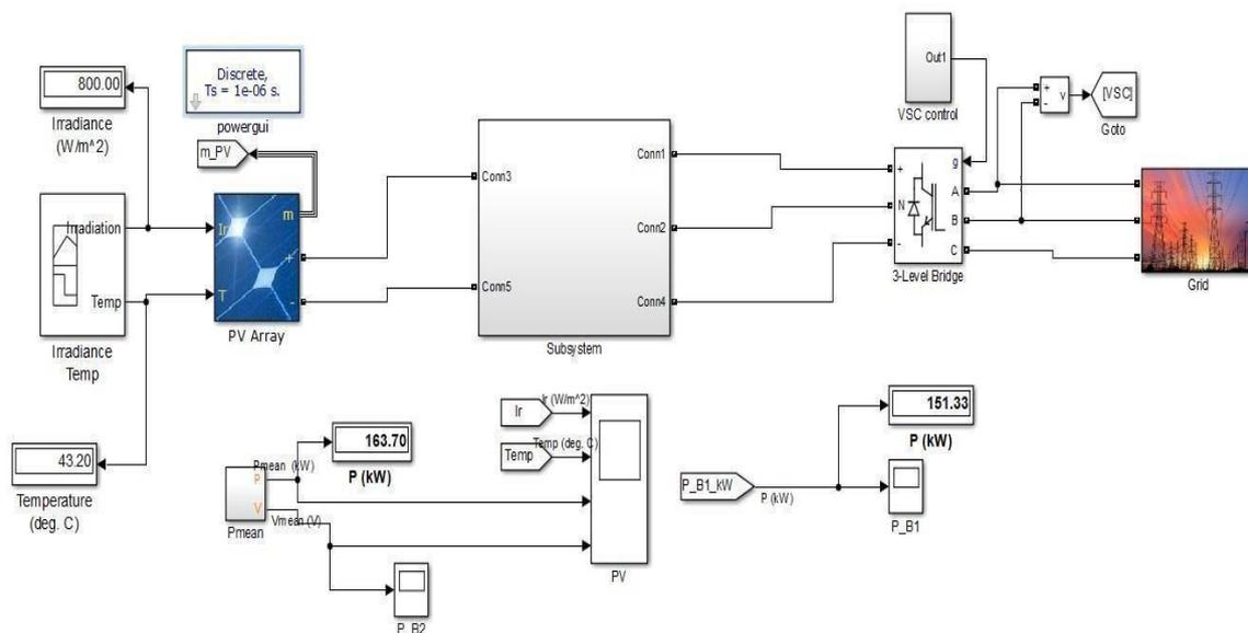
Fig 4. Simulation model of grid connected PV array by using Z-source converter
