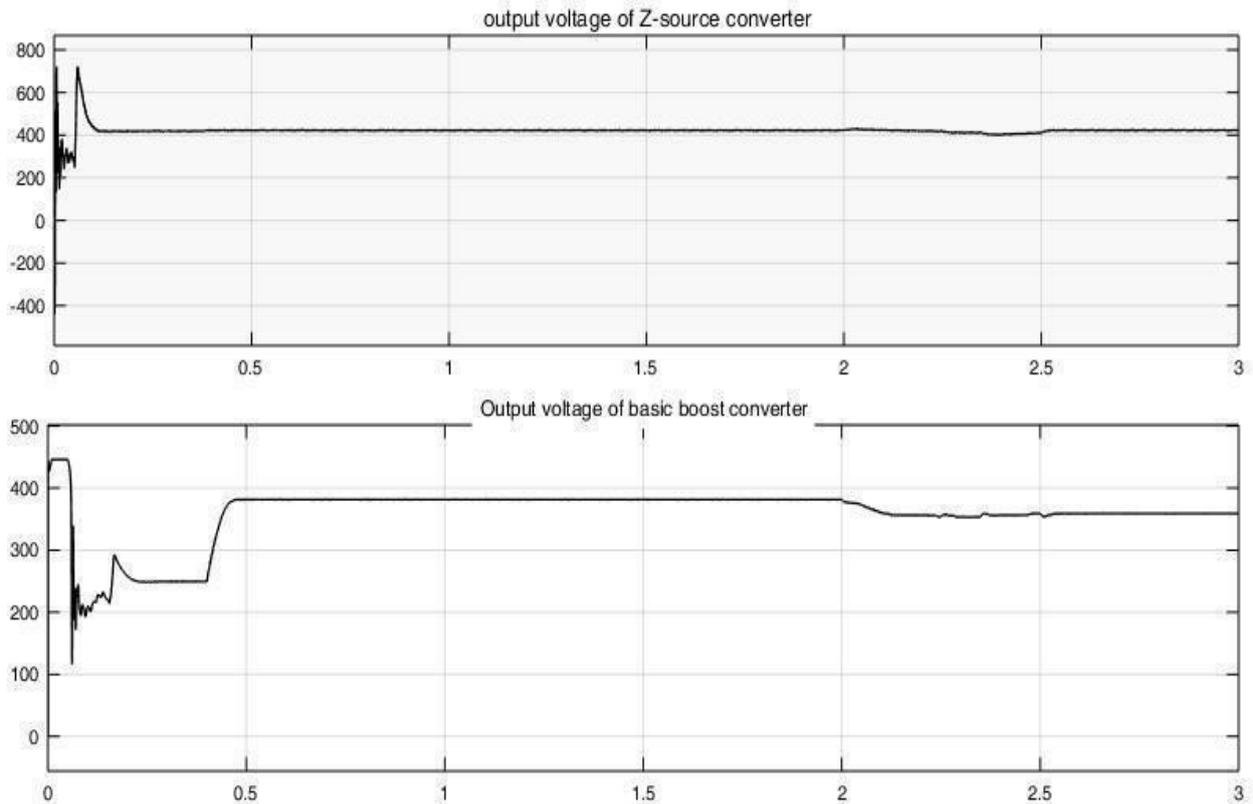
Fig 7:- PV mean output voltage by using Z-source and boost converter
