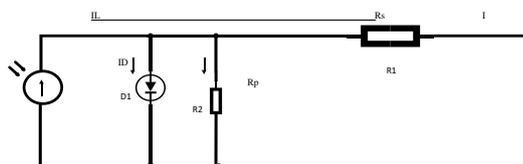
Fig2. Equivalent circuit of solar PV cell
